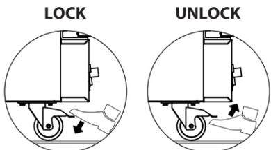
Using your foot, press down on the caster's pedal to lock the oven in place. Lift up on the bottom of the pedal to unlock the caster to reposition or move the oven.
