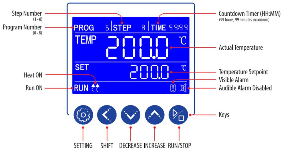
**PROG Area:** Displays the program working or setting group. Controller is capable of programming and storing up to 7 programs.
