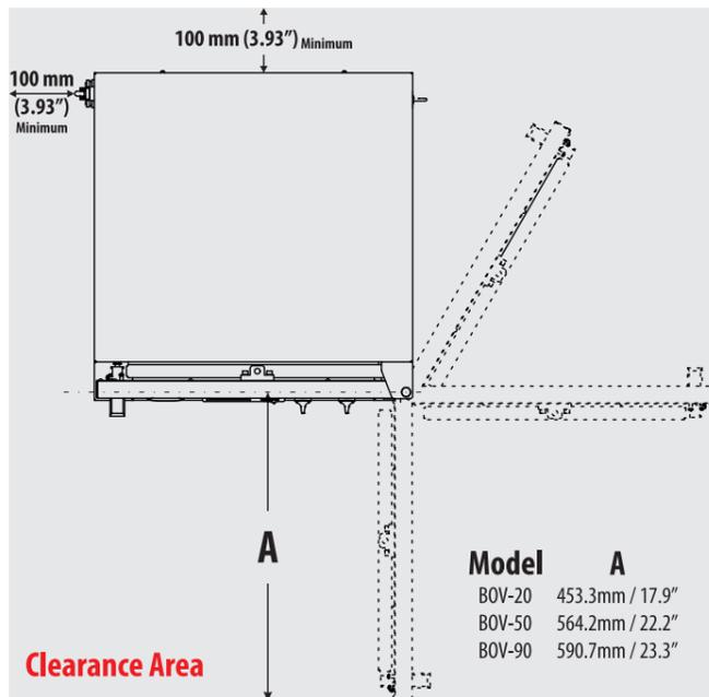
Position the vacuum oven on the floor or a work surface strong enough to carry the oven's weight.
