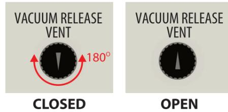
Rotate the vacuum release vent knob 180° to relieve the vacuum applied at the factory prior to shipping. Upon relieving the applied vacuum, close the vent.
