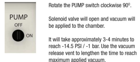
**!** It is not required to draw a vacuum to apply heat to the specimens in the oven. However, applying a vacuum first will reduce the humidity in the oven and increase the speed to reach desired temperature.
