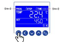
Press the SETTING key to accept temperature setpoint. The first TIME digit will blink.
