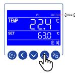
Press the INCREASE or DECREASE key to change the first digit. Press the SHIFT key to move to the second digit. Digit will blink. Press the INCREASE key to enter the second digit. Continue until parameter is set.
