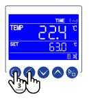
Press the SETTING and SHIFT keys for 3 seconds to enter the controller's internal parameter settings.
