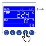
Press the INCREASE key to enter the first cycle value. Press the SHIFT key to move to the second cycle digit. Digit will blink. Press the INCREASE key to enter the second cycle
