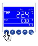
Press the SETTING key 4 times to set parameter Po and return to standard state.
