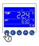
Press the SETTING key 2 times to set parameter CF and return to standard state.
