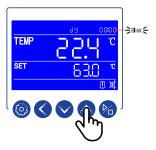
Press the INCREASE key to enter the first time value. Press the SHIFT key to move to the second time digit. Digit will blink. Press the INCREASE key to enter the second time value.
