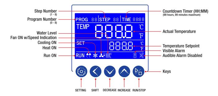
PROG Area: Displays the program working or setting group. Controller is capable of programming and storing up to 8 programs.
