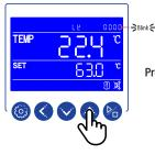
Press the SETTING key to enter Level 1 parameters.
