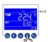
Press the INCREASE key to change the first digit. Press the SHIFT key to move to the second digit. Digit will blink. Press the INCREASE key to enter the second digit. Continue until parameter is set.
