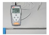
Upon reaching the set temperature, insert thermometer probe into the test hole.
