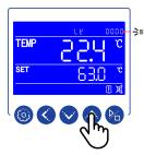
Press the INCREASE key to enter the first code digit. Press the SHIFT key to move to the second code digit. Digit will blink. Press the INCREASE key to enter the second code digit.
