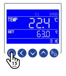
Press the SETTING key 11 times to scroll through parameters until the parameter CF appears.
