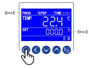
Pressing the SETTING key starts the programming process.
