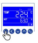
Press the SETTING key 1 time to set parameter Mo and return to standard state.
