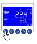
Press the SETTING key to enter the Level 2 controller parameters.
