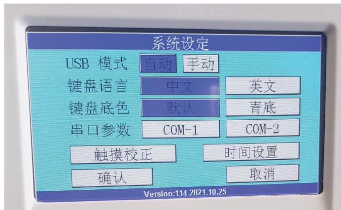
This screen can appear upon powering up the BOF or BON oven, potentially due to the operator touching the screen during power-up.
