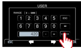
Enter the number of delay minutes using the keyboard. Maximum number of delay minutes is 5999.
