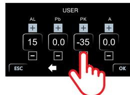
Set the desired Pb and PK parameters by pressing the + or - key for each digit.
