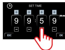
**Generation 1 & 3:** Set the desired time by pressing the + or – button for each digit. Maximum run time is 99:59.
