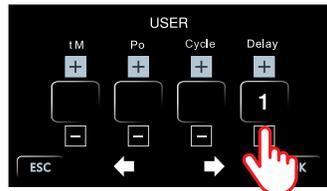
Set the number of cycles by pressing the + or – button for each digit. Maximum number of delay minutes is 5999.
