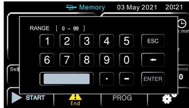
Figure 4.7. Setting time (hours) for fixed-value programs. Generation 2.
