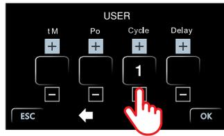
Set the number of cycles by pressing the + or - button for each digit. Maximum number of cycles is 99.
