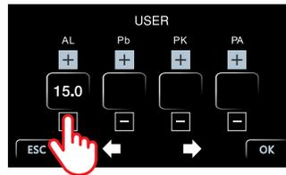
Set the alarm (AL) value by pressing the + or – button for each digit. Maximum alarm value is 100.0.
