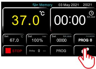
Press the Operational Settings (gears) button in the lower right corner of the home screen.
