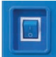
**Generations 2 & 3:** Ensure the circuit breaker's lever is in the up position. Then, push the power switch on the bottom left side of the unit.
