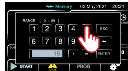
**Generation 2:** Set the desired run time by using the keyboard. The time is split into hours and minutes. Each has a keyboard for setting.
