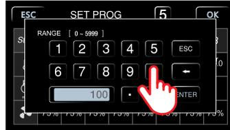
Set the run time using the keyboard. The maximum run time is 5999 minutes.
