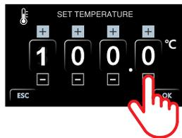
**Generation 1 & 3.** Set the desired temperature by pressing the + or – button for each digit.
