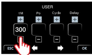
Press the PLUS (+) or MINUS (-) button if the tM parameter needs correction. Press and hold to rapidly cycle to the maximum temperature required.
