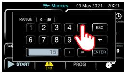
**Generation 2:** Enter the run time using the keyboard. Maximum run time (minutes) is 59.
