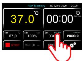
Press the left side of the RUN time button to set hours (hh) or right side to set minutes (mm).
