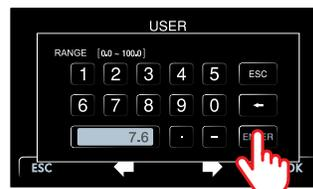
Enter the alarm (AL) value using the keyboard. Maximum alarm value is 100.0.
