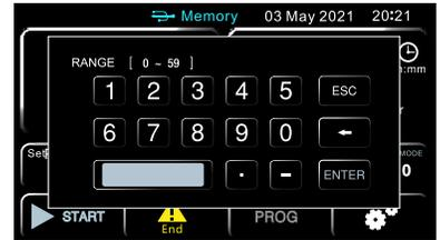
Figure 4.8. Setting time (minutes) for fixed-value programs. Generation 2.
