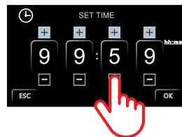
**Generation 1 & 3:** Set the desired time by pressing the + or - button for each digit. Maximum run time is 99:59.
