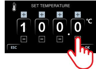
**Generation 1 & 3.** Set the desired temperature by pressing the + or – button for each digit.
