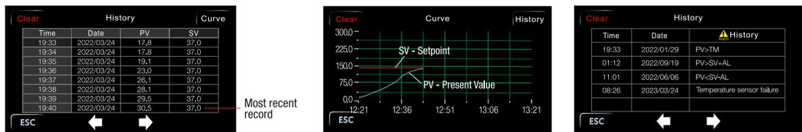
Temperature-related data is viewable in two formats: table and curve. The alarm history data is presented in a table format. For more details see Sections 6.2.2, 6.2.3, and 6.2.4.
