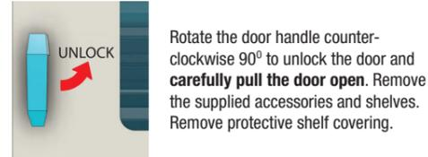
Rotate the door handle counter-clockwise 90° to unlock the door and carefully pull the door open. Remove the supplied accessories and shelves. Remove protective shelf covering.
