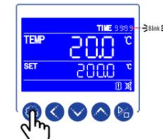
Press the SETTING key to accept temperature setpoint. "End" in TIME area will change to run time digits. First digit will blink.
