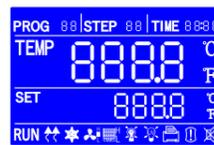
Upon turning the unit's power on, the controller will cycle through these two start-up screens.
