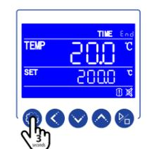
Upon setting the run time, press and hold the SETTING key for 3 seconds to complete the program.
