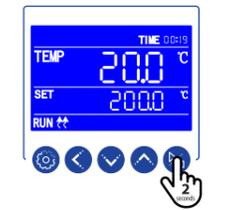
Pressing the RUN key for 2 seconds starts the program. RUN, HEAT, and run time illuminate.
