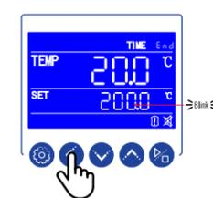
Press the SHIFT key to move to the next parameter digits. Each move will cause parameter to blink.
