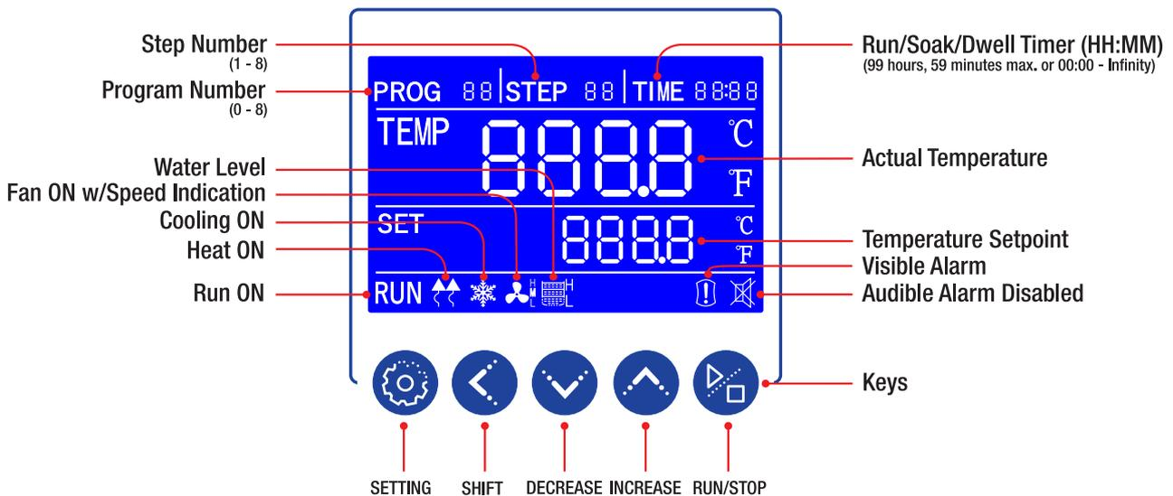
**PROG Area:** Displays the program working or setting group. Controller is capable of programming and storing 1 fixed value program and up to 8 multi-step programs.
