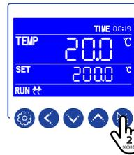
Pressing the RUN key for 2 seconds starts the program. RUN, HEAT, and run/soak time illuminate.
