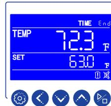
Upon changing the temperature unit of measurement, the present value (PV) temperature will change its value.
