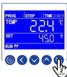
Pressing the RUN key for 2 seconds starts the program. STEP area, RUN, HEAT, and run/soak time illuminate.
