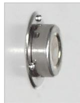
The test hole / accessory port is Ø25mm and located on the right side of the incubator.
