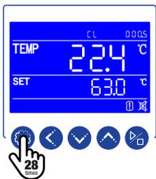
Press the SETTING key 28 times to scroll through parameters until the parameter Li appears.
