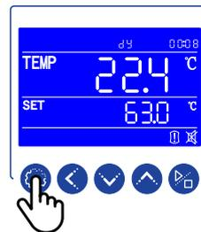
Press the SETTING key 1 time to set parameter dy and return to fixed value program the home screen.
