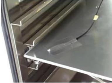
Use high-temperature tape, preferably aluminum tape, to attach the thermocouple to the **geometric center** of one shelf.
