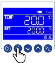
Press the SHIFT key to move to the next parameter digits. Each move will cause parameter to blink.
