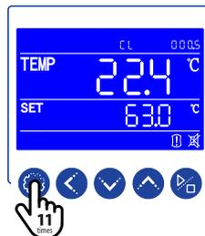
Press the SETTING key 11 times to scroll through parameters until the parameter Ht appears.
