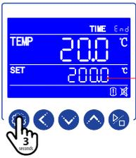
Pressing the SETTING key for 3 seconds, starts the programming process.
