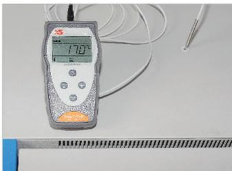
Upon reaching the set temperature, insert thermometer probe into the test hole.
