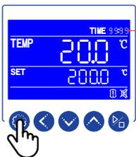
Press the SETTING key to accept temperature setpoint. "End" in TIME area will change to run/soak time digits. First digit will blink.
