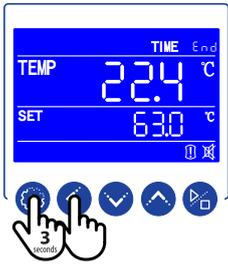
Press and hold SETTING and shift keys for 3 seconds to view the controller's operational parameters.
