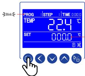
Pressing the SETTING key starts the programming process.
