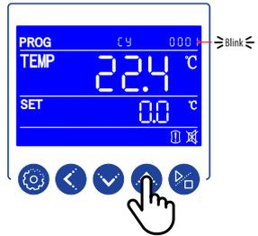
Press the INCREASE key to enter the first cycle value. Press the SHIFT key to move to the second cycle digit. Digit will blink. Press the INCREASE key to enter the second cycle value.
