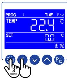
Press the SETTING and SHIFT keys for 3 seconds to enter the controller's operational parameter settings. Time area will change and first digit will blink.
