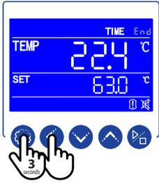
Press the SETTING and SHIFT keys for 3 seconds to enter the controller's operational parameter settings.
