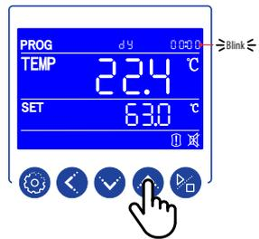
Press the INCREASE key to enter the first time value. Press the SHIFT key to move to the second cycle digit. Digit will blink. Press the INCREASE key to enter the second time value.
