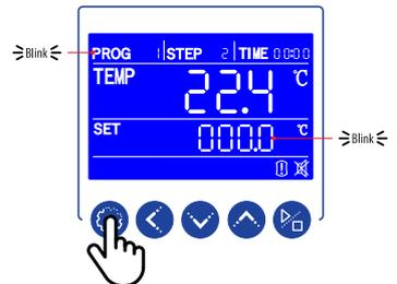
Press the SETTING key to accept the run/soak time.
