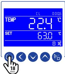
Press the SETTING key 18 times to scroll through parameters until the parameter CF appears.
