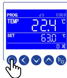
Press the SETTING key 1 time to set parameter dy and return to multi-step program home screen.
