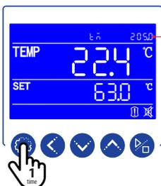
The tM parameter will appear. Press the SETTING key 2 times to scroll through parameters until the parameter AL appears.
