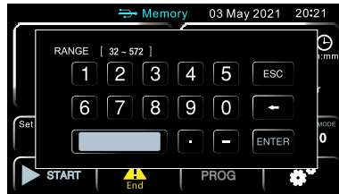
Figure 4.4. Setting temperature for fixed-value programs. Generation 2; Fahrenheit. When in Celsius the range changes to 0 - 300. The set temperature cannot be greater than the high-end of the range.
