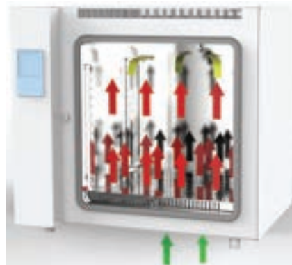
Figure 2.10. The dark green arrows show ambient air. The red show heated air circulating in the chamber while the light green arrows show the exhaust air exiting the chamber.
